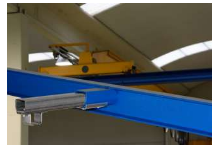
BEAM WELDED SUPPORT
