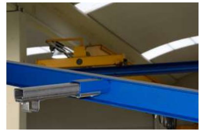
BEAM WELDED SUPPORT
