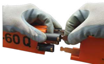
Insert the ends of the copper conductors into the spring connectors one by one approx. 5-10 mm.
